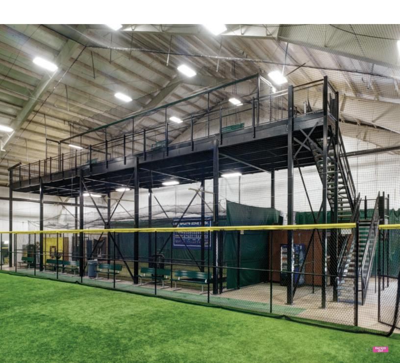
Cogan industrial catwalk mezzanines improve in-plant circulation and provide secure work platforms for overhead maintenance.
